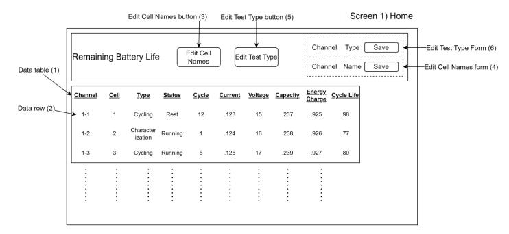
The Home screen is what is displayed when a user first opens our site. It provides a dashboard overview of the tests being run in the Neware battery tester. It allows users to view the status of their tests and monitor the progress of all channels simultaneously.
