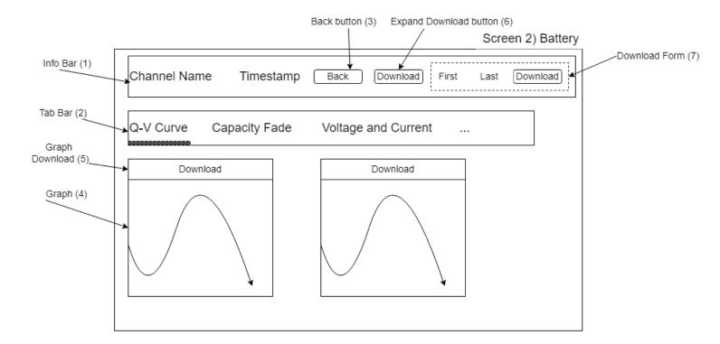
The Battery screen is what is displayed when a user clicks a row on the Home page and is navigated to the Battery page for the clicked-on row. It displays more detailed information about the cell running in the particular channel by displaying graphs of its real-time and historical data
